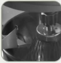
Bowl guard of transparent AR plastic and conveyor for liquid addition.
